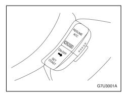
The cruise control pad is located on the right side of the steering wheel.
